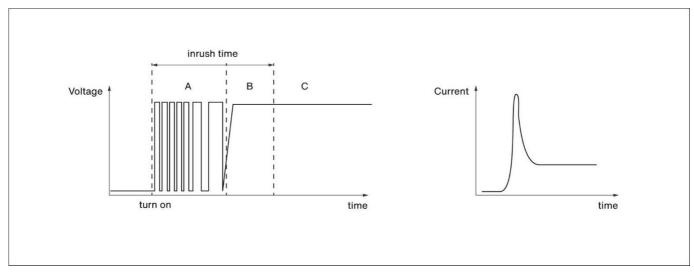
Figure 19: Capacitive soft start
