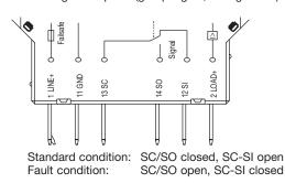
ESX10-S115 with signal input IN+ with signal output F (group signal, N/O)
