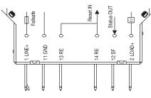
Standard condition: SF +24V = OK Fault condition: SF 0V
